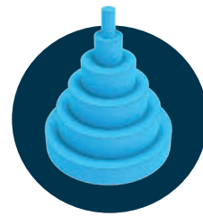
DIMENSIONAL ACCURACY TEST: Probes a printer's ability to fabricate dimensionally correct geometries in the XY plane. Reveals backlash in X and Y directions if present.
