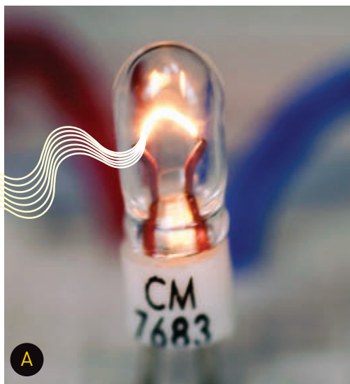
Chicago Miniature Lamps part #7683. 5V, 60mA, rated 25,000 hours.
