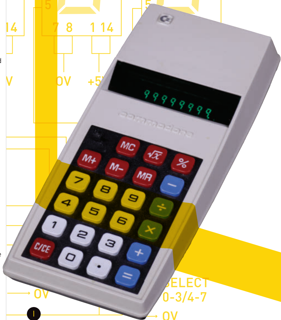
Don't think of it as a piece of old junk. Think of its vacuum fluorescent display becoming an eye-catching output device for a microcontroller.
